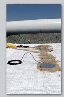
To scale the tensile strength in the grid and the loading pressure under the reinforced working platform, strain gauges were applied on the Combigrid® layer and on load-bearing measurement plates in the subsoil under the reinforcement. These tools enabled the collection of exact stress conditions in the geogrid and in the reinforced base course during different stages of the construction process.
